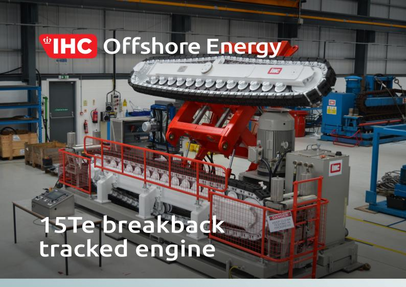
Our 15Te tracked tensioners are suitable to be operated in the most hazardous environments the industry has to offer. With its robust design, which has been developed by Royal IHC over the past 20 years, this is a reliable system for the laying and retrieval of subsea cables and umbilical.
